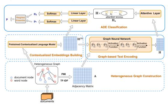
Figure 1: The illustration of the model architecture with contextualized graph embeddings for ADE detection
