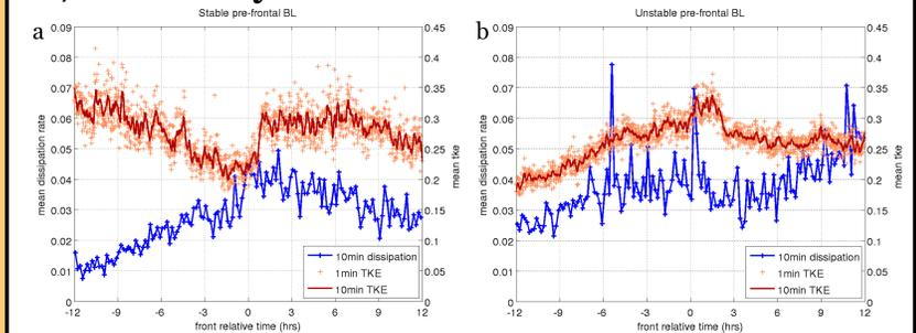
Fig.6. Composite of TKE and  $\epsilon$  across cold fronts for fronts which had a (a) stable and (b) unstable pre-frontal boundary layer. Stability was determined by averaging (z-d)/L for the 3 hours before the front was observed. An average (z-d)/L > 0.1 was classified as stable and (z-d)/L < -0.1 was classified as unstable.
