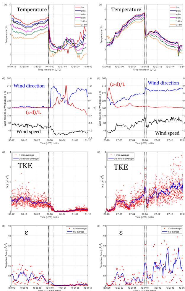
Fig.3. Observations of a cold front on 30 Oct 2007. (a) Temperature, (b) wind speed and direction and (z-d)/L, (c) TKE and (d)  $\epsilon$ . Vertical dashed lines indicate the frontal zone
