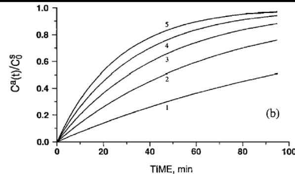
**Figure 4.** Behavior of a closed chamber with a  $V/A$  ratio of 20 cm when measuring gases with different  $D^a$ . For curves 1, 2, 3, 4, and 5 the  $D^a$  values are 0.05, 0.10, 0.15, 0.20, and 0.25  $\text{cm}^2 \text{s}^{-1}$ , respectively.
