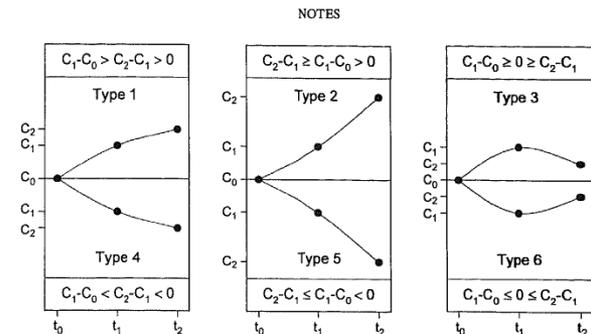
Fig. 1. The defining inequality and an example of each of the six possible curve shapes for N<sub>2</sub>O accumulation in a non-steady-state chamber during two successive equal periods beginning with chamber deployment.
