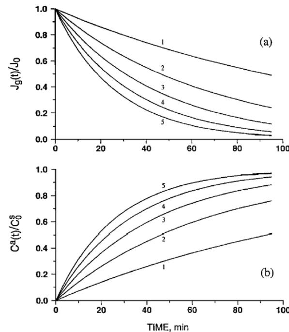
**Figure 4.** Behavior of a closed chamber with a  $V/A$  ratio of 20 cm when measuring gases with different  $D^a$ . For curves 1, 2, 3, 4, and 5 the  $D^a$  values are 0.05, 0.10, 0.15, 0.20, and 0.25  $\text{cm}^2 \text{s}^{-1}$ , respectively.
