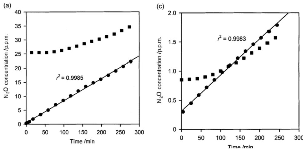
**Figure 3** Measured changes in N<sub>2</sub>O concentrations below the source of N<sub>2</sub>O production (■) and in the headspace (●) of soil core for (a) wet core with low air-filled porosity; (b) core at intermediate air-filled porosity; (c) relatively dry soil core. A linear regression (continuous line) has been fitted to the headspace concentration over time.
