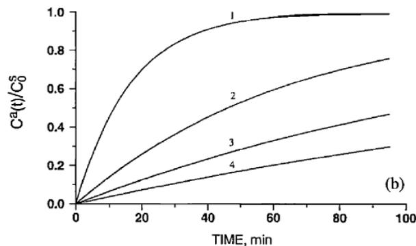
**Figure 3.** Behavior of shallow closed chamber with different  $V/A$  ratio ( $H$ ). For curves 1, 2, 3, and 4 in the figure the  $V/A$  ratios are 10, 20, 30, and 40 cm, respectively.
