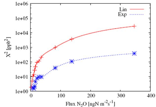
Fig. 7 Goodness-of-fit ( $\chi^2$ ) of linear and exponential regression method to  $N_2O$  automatic chamber measurements as a function of the  $N_2O$  flux. Data points represent the average goodness-of-fit and average  $N_2O$  flux over a bin including hundred  $N_2O$  fluxes
