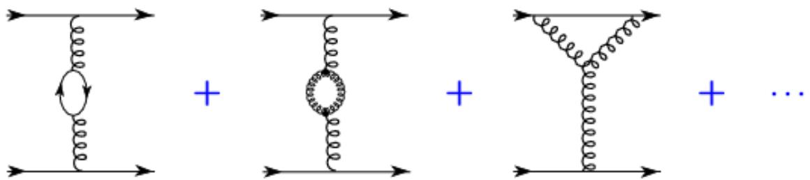
$$\alpha_s(Q^2) = \frac{\alpha_s(Q_0^2)}{1 - \beta_1 \frac{\alpha_s(Q_0^2)}{2\pi} \ln \left( \frac{Q^2}{Q_0^2} \right)}$$
