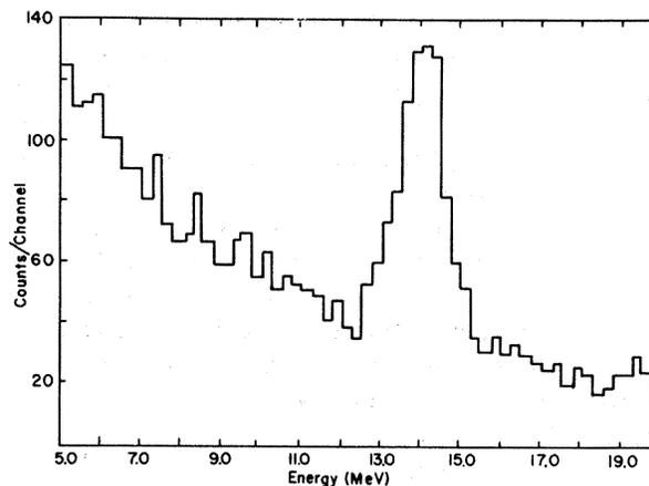
FIG. 1. Typical pulse-height spectrum from a 5-mm-thick solid-state detector. The elastic peak appears at an energy of  $14.1 \text{ MeV}$  and is due to protons stopping in the detector.
