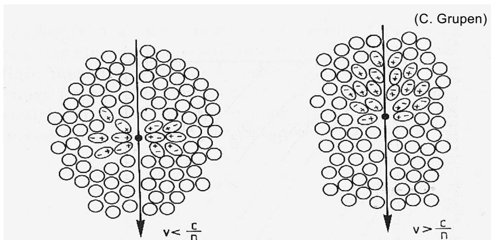
Fig. 6.7. Illustration of the Cherenkov effect [68].
