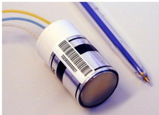
used by e.g. CMS for readout of endcap calorimeter (also already DELPHI & OPAL at LEP used same technology)
