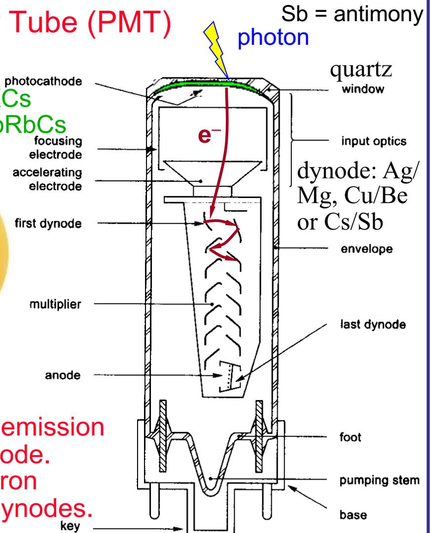
PMT's very sensitive to magnetic fields, even to earth field (30-60  $\mu\text{T}$ ).
