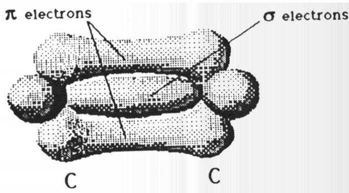
Scintillation based on the two “ $\pi$ ” electrons of the C–C bonds in “aromatic rings” like benzene.
