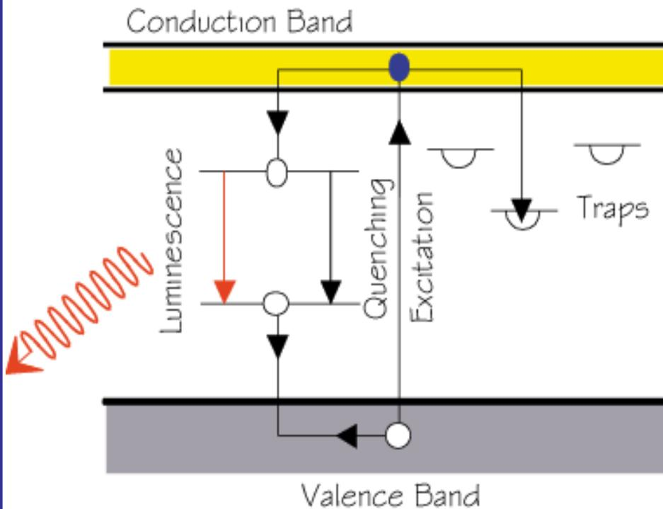
energy bands in crystals activated by impurity traces, often  $\geq 2$  time constants:
