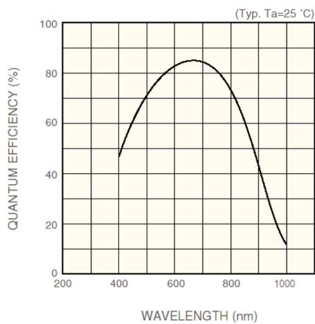
multi-pixel photon counters (MPPCs) (for new TOTEM T2) & single SiPMs
