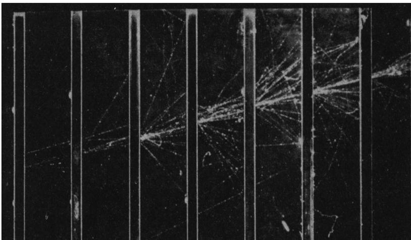
Electron shower in a cloud chamber with lead absorbers
