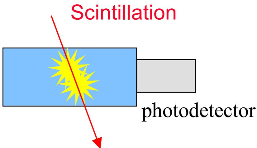
Energy deposition by ionizing particle → excited molecules → small fraction of energy released as optical photons (scintillation light or luminescence)
