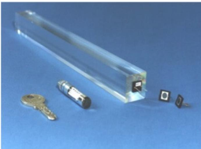
A lead tungstate (PbWO<sub>4</sub>) crystal for the CMS electromagnetic calorimeter. PbWO<sub>4</sub> has fast signal, high density & good radiation tolerance at reasonable cost. Only disadvantage is relatively low light yield.
