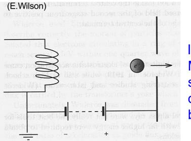
limited to ~ a few MeV (even in staged approach) due to electrical breakdown
