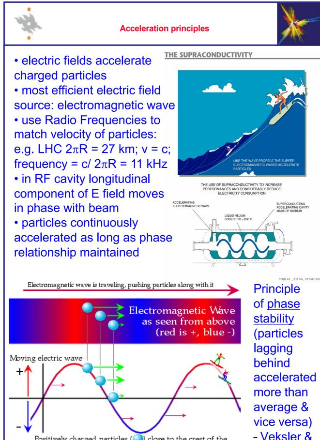
Positively charged particles () close to the crest of the E-M wave experience the most force forward; those closer to the center experience less of a force. The result is that the particles tend to move together with the wave.
