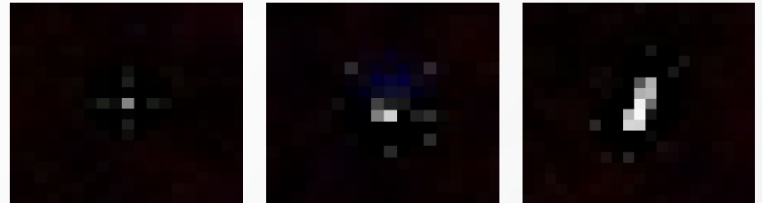
Gamma particles of varying energies from Ba-133
