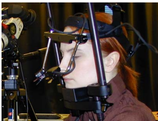
Figure 4. A test subject with head-mounted gaze tracking system.
