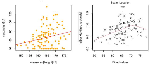
In the left-hand plot, we see that in the new data, the variance increases with height. In the right-hand plot, we see an increasing pattern in the standardized residuals, which indicates that the variance of residuals is changing as a function of the fitted values. This violates the assumptions of the linear regression model.
