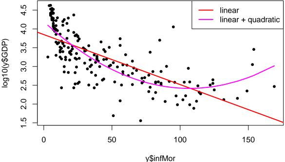
This quadratic term clearly improves model fit (R2 increases from 50% to 62%) and the fitted values take into account the curved pattern in the data. Let's see the diagnostic plots.
