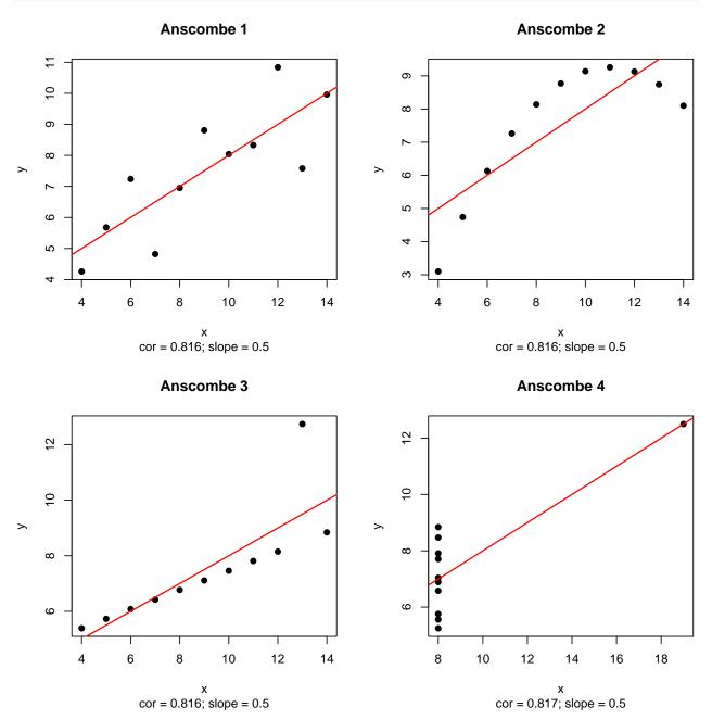
We see that the data sets are identical with respect to the x-y correlation and the linear model slope, but we also see that the data sets are very different in other respects, and, in particular, the linear model does not seem an appropriate description of the X-Y relationship for the data sets 2, 3 and 4.
