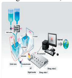
Fig. 1: Schematic diagram of the remote interactive real experiment across Internet – Electrochemical cell (with two vessels and two metallic electrodes connected via a membrane, the measured data is the voltage of the conductivity of the electrolyte and its pH factor)
