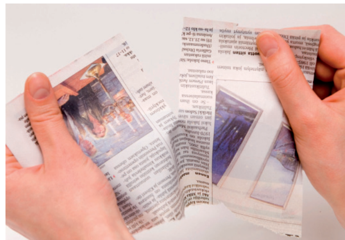
During paper production, the cluster fibres get a parallel orientation. This is the reason why newspaper paper behaves in a different way when torn vertically and horizontally.
