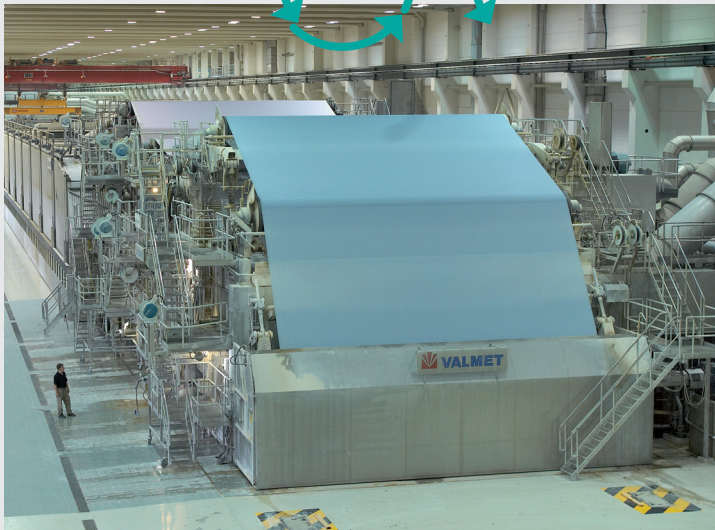
Paper sheet formation in a paper-making machine.
