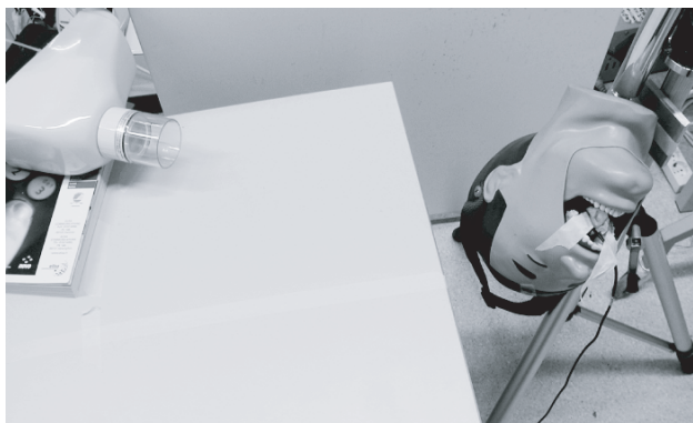
FIG. 5.7. Left: Geometry for intraoral measurements. The detector is in fixed position inside the patient's mouth. The source locations are denoted by black dots (7 projections from a total view-angle of 60^\circ ). Right: Experimental setup.
