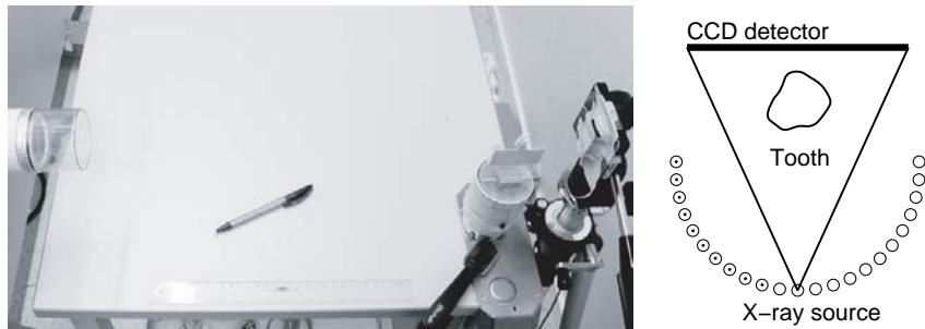
FIG. 5.3. Left: The experimental setup. The X-ray source is on the left and the detector is attached to the camera stand on the right. The tooth phantom is positioned on the rotating platform. Right: Illustration of the projection geometry. Circles denote the source locations for the full-angle data (23 projections from total view-angle of 187^\circ ). The projections used in limited angle computations (10 projections from view-angle of 76^\circ ) are denoted by black dots within the circles. For clarity, the location and alignment of the detector with respect to the source is depicted only for one source location.
