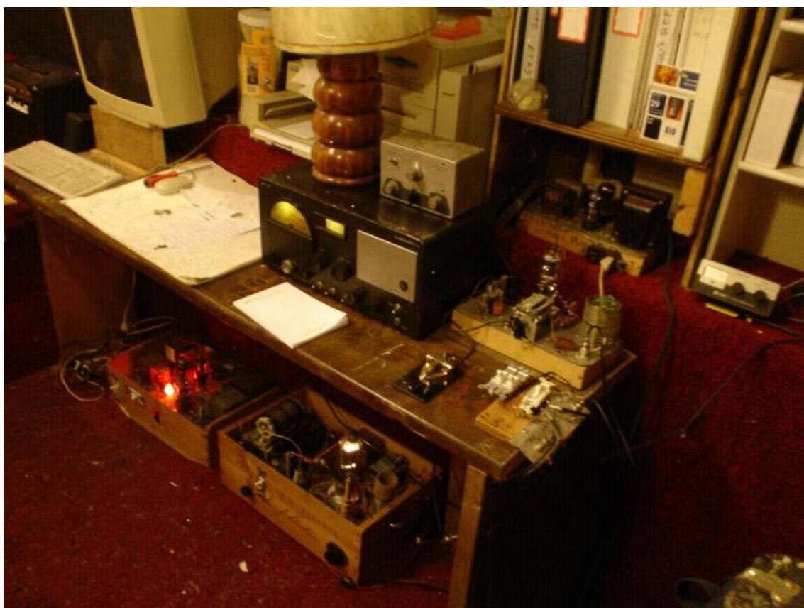
To properly give "assistance" to my 1955 novice station, I have included under the operating table a microwave transformer power supply and a single 810 final amplifier, which by the way, does a really good job of assisting.
