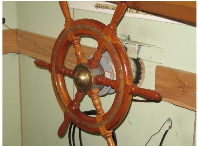
Armstrong rotating system of the 42 m high tower. (OH1WZ).
