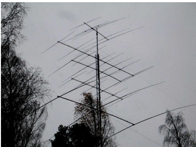
The 42-m rotating tower from 1982 hosts (top → down) a WRTC2002-tribander with a rotator, a 6-el yagi for 21 MHz, a 4/4-el yagi pair for 14 MHz, a 6-el yagi for 28 MHz and a full-size 3-el yagi for 7 MHz. The tallest pines are 25 m high now in 2006. (OH1WZ).
