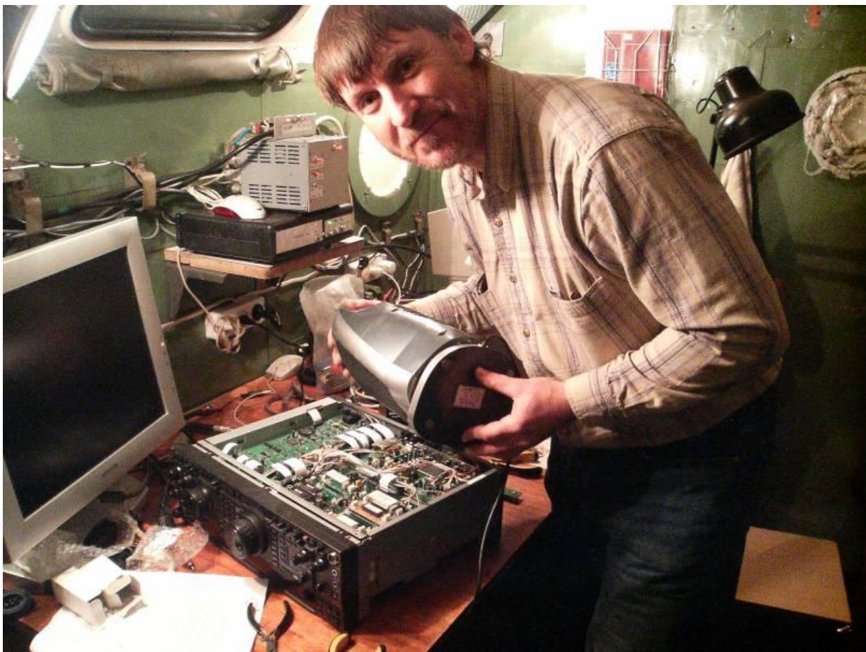
Mike, RW0CN was the host for Marko, N5ZO (RW0CWA) in CQ WW CW 2008. The radio is warmed up to allow the installation of some tight-fitting filter-units.
