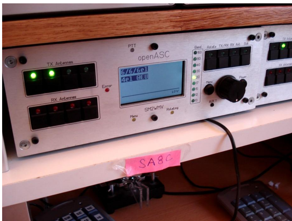
openASC - Box controlling the whole station, from ant-combinations to rotation of 4-SQ or the towers.
