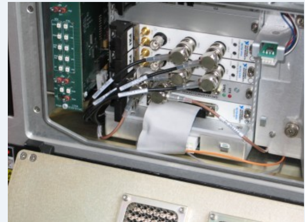
1. Leica ALS60, GPS/IMU & electronics. 2. Oscilloscopes for the AD conversion
