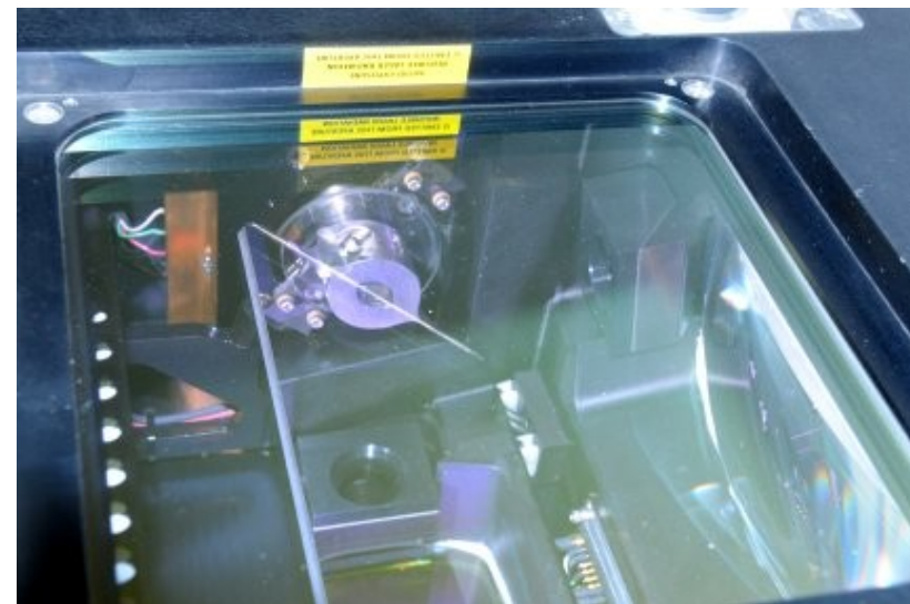
Aperture of an ALS50-ii sensor. Oscillating mirror in resting position, collimating lens on the right.
