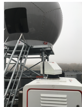
Figure: X-band radar and Doppler lidar at the measurement site. Photo by Raisa Lehtinen.
