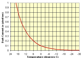
Effect of Temperature on Dark Current
