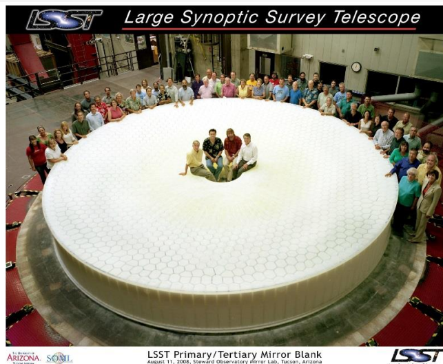
LSST Primary/Tertiary Mirror Blank August 11, 2008, Steward Observatory Mirror Lab, Tucson, Arizona
