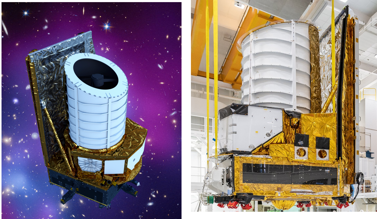
Figure 43: Left: Artist view of Euclid. Credit: ESA/ATG medialab (spacecraft); NASA, ESA, CXC, C. Ma, H. Ebeling and E. Barrett (University of Hawaii/IfA), et al. and STScI (background). Right: Euclid in a clean room of Thales Alenia Space in March 2023 before shipping to the launch site. Euclid is 4.7 m tall and 3.7 m in diameter and has a mass of 2 tonnes. Credit: Thales Alenia Space.
