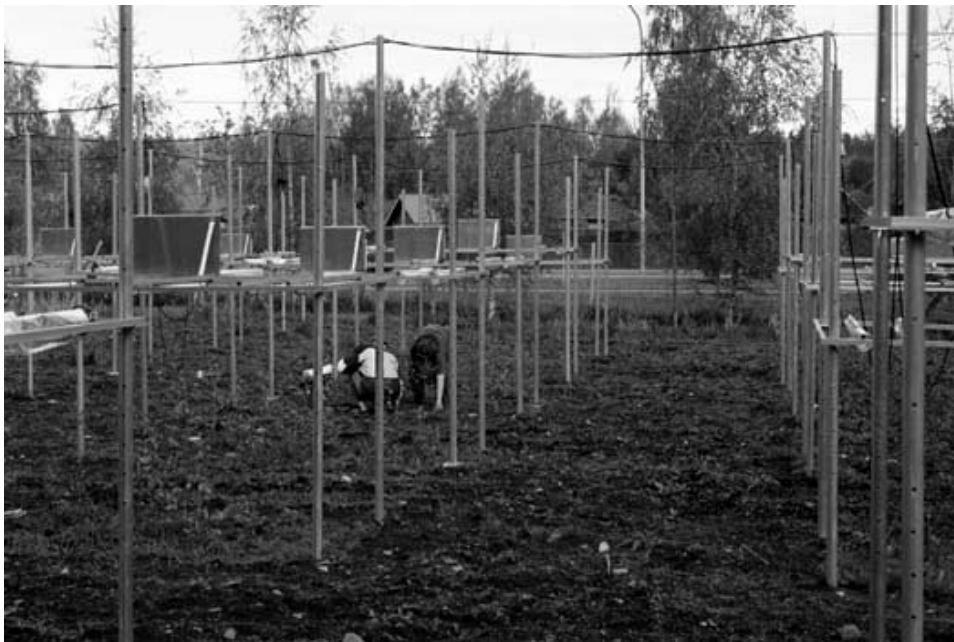
Figure 1: Partial view of the modulated UV-B supplementation system in Joensuu. Two years old birch seedlings growing under the frames.
