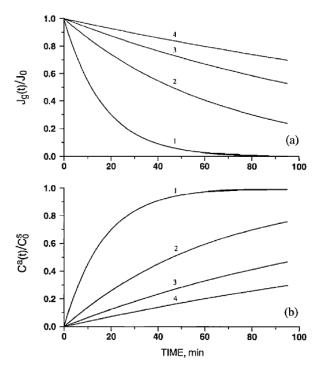
**Figure 3.** Behavior of shallow closed chamber with different V/A ratio (H). For curves 1, 2, 3, and 4 in the figure the V/A ratios are 10, 20, 30, and 40 cm, respectively.
