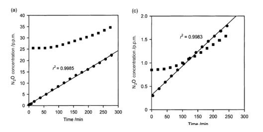
Figure 3 Measured changes in N<sub>2</sub>O concentrations below the source of N<sub>2</sub>O production ( $\blacksquare$ ) and in the headspace ( $\bullet$ ) of soil core for (a) wet core with low air-filled porosity; (b) core at intermediate airfilled porosity; (c) relatively dry soil core. A linear regression (continuous line) has been fitted to the headspace concentration over time.
