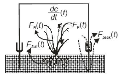
Fig. 1. Schematic of the CO<sub>2</sub> fluxes in the chamber headspace which make up to the net CO<sub>2</sub> flux  $F_{net}$  (details in the text, Eq. (1)).  $F_{Soil}(t)$  is the diffusive efflux from the soil,  $F_P(t)$  is photosynthesis,  $F_R(t)$  is aboveground plant respiration,  $F_{Leak}(t)$  is leak flux. dc/dt(t) is the CO<sub>2</sub> concentration change over time t in the chamber headspace.
