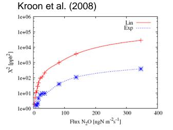
Fig. 7 Goodness-of-fit  $(\chi^2)$  of linear and exponential regression method to N<sub>2</sub>O automatic chamber measurements as a function of the N<sub>2</sub>O flux. Data points represent the average goodness-of-fit and average N<sub>2</sub>O flux over a bin including hundred N<sub>2</sub>O fluxes
