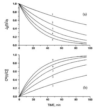
Figure 4. Behavior of a closed chamber with a V/A ratio of 20 cm when measuring gases with different  $D^a$ . For curves 1, 2, 3, 4, and 5 the  $D^a$  values are 0.05, 0.10, 0.15, 0.20, and 0.25 cm<sup>2</sup> s<sup>-1</sup>, respectively.
