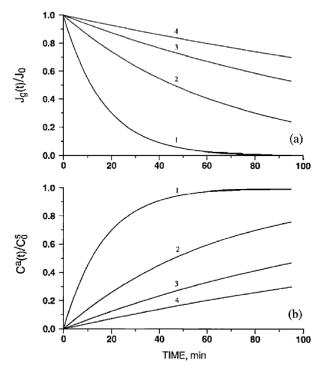
**Figure 3.** Behavior of shallow closed chamber with different V/A ratio (H). For curves 1, 2, 3, and 4 in the figure the V/A ratios are 10, 20, 30, and 40 cm, respectively.
