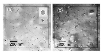
FIG. 1. In situ TEM bright field images of Co nanoparticles on Cu(100) at 300 K (a) and at 600 K (b). The images show representative areas of the samples used for the AFM scans in Fig. 2. The particle coverage is identical within 5%. The insets show enlargements of typical clusters.
