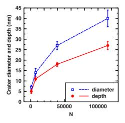
FIG. 2. (Color online) Crater diameter and depth at different cluster sizes N. Diameter grows faster than depth at large N.
