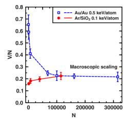
FIG. 1. (Color online) Ratio of crater volume and cluster size V/N as a function of cluster size N. Horizontal line means that the volume increases linearly with the impactor size, which is typical to macroscopic impacts. The values for the Au impact are from Ref. 9.
