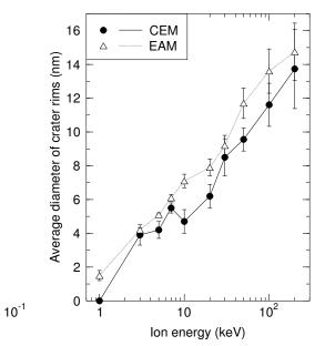
Fig. 10. Average maximum diameter of crater rims as a function of ion energy. Only clearly visible craters are included in the averages.
