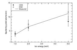
Fig. 4. Comparison of experimental and simulated average sputtering yields of gold atoms from the Au(111) surface bombarded by Ar ions. The experimental values are from Ref. [73,74]
