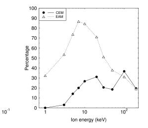
Fig. 5. Percentage of crater events out of all simulated events at different ion energies. The results are based on analysis of crater volumes and confirmed by visual inspection of simulations.
