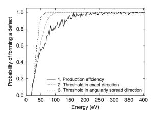
Fig. 2. Probability to form a defect at a given energy calculated in three different ways (see text) with the ABC potential.
