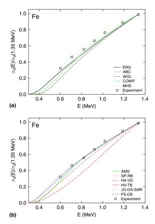
Fig. 5. Atom displacement cross sections  $\sigma_d(E)$  normalized to the value at 1.35 MeV, as a function of average electron beam energy *E*. The squares show experimental data from [13]. The lines show theoretical results obtained by converting MD simulations of defect formation probability  $N_{\rm FP}(T)$  into displacement cross sections using the McKinley–Feshbach equations (see text) [56]. For clarity the figure is split in two parts.
