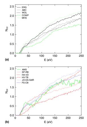
Fig. 4. Average number of defects produced as a function of recoil energy  $N_{\rm FP}(T)$  for the different potentials. For clarity the figure is split in two parts.
