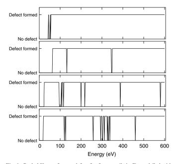
Fig. 1. Probability to form a defect for four recoils in Fe modelled with the ABC potential, as a function of recoil energy. Note that the data illustrates specifically the probability to form *at least* one defect; at the higher energies in many cases more than one defect is formed. In each of the four cases the initial state of the simulation is identical, including identical thermal atom displacements, except for the initial ion energy which is raised in steps of 2 eV.
