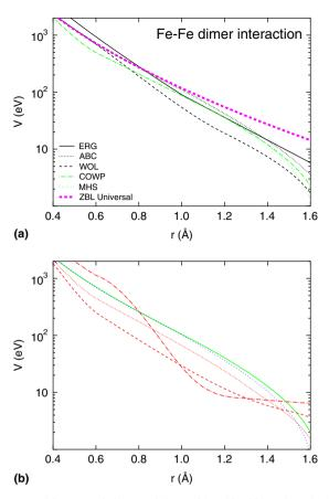
Fig. 3. Repulsive part of all potentials considered in this study, calculated as the total for an  $Fe_2$  dimer. The potential abbreviations and references to them are given in the text. For clarity the figure is split in two parts.
