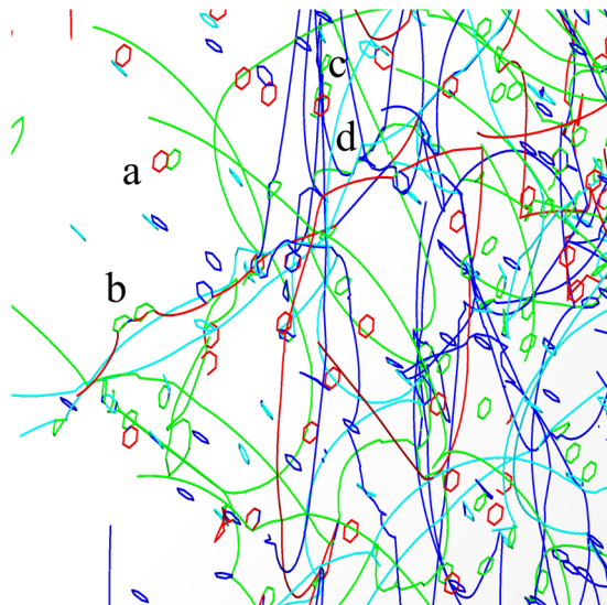
Figure 5. Close-up view of the 3D structure of a dislocation system with glissile dislocation loops at a strain of \varepsilon = 0.5\% . Different Burgers vectors are indicated with different colors as follows: dark blue b = \frac{1}{2}\langle 111 \rangle , cyan b = \frac{1}{2}\langle 11\bar{1} \rangle , green b = \frac{1}{2}\langle \bar{1}11 \rangle , and red b = \frac{1}{2}\langle 1\bar{1}1 \rangle . Continuous dislocations and loops evolve into a complex network where they pin to each other. a) Loop dipole b) dislocation pinned by loops c) loops decorating a dislocation d) complex junction. The loop radius is r_l = 5 nm.
