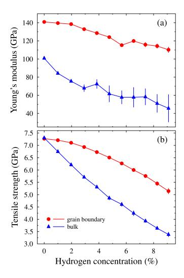
Figure 4: (a) Young's modulus  $E = \sigma_{zz}/\varepsilon_{zz}$  and (b) the tensile strength  $\sigma_{\rm TS}$  as functions of the atomic hydrogen concentration for bulk bcc iron (triangles) and for the grain-boundary system (circles). The error bars are calculated as the standard deviation of ten simulations. The lines are guides to the eye.
