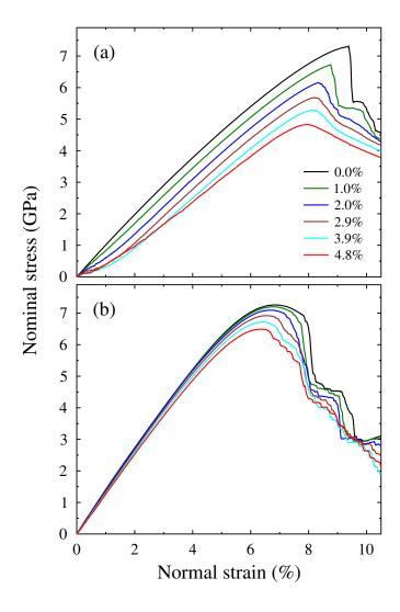
Figure 2: Uniaxial nominal stress  $\sigma_{zz}$  as a function of normal tensile strain  $\varepsilon_{zz}$  for (a) monocrystalline bulk iron and (b) an iron bicrystal with a symmetric tilt boundary (Fig. 1). The legend shows the atomic hydrogen concentration for each curve. Uniaxial tension is exerted along the z axis, perpendicular to the grain-boundary plane.
