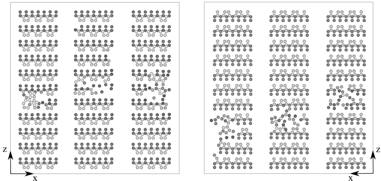
FIG. 3. Examples of damage to the first two atomic layers on the surface of the wire where the ion enters (left) and the bottom of the wire where the ion exits (right). The extent of the damage is usually limited to a couple unit cells in both dimensions. Coloring is by distance from the core of the wire, with dark being closer to the core.
