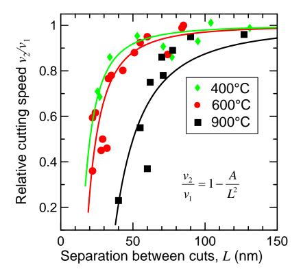
Figure 2. Relative cutting speed  $v_2/v_1$  at various temperatures as a function of separation between the cuts L. Symbols stand for the experimental data, solid lines are fits obtained with Eq. (4). All curves were scaled to  $v_1 = v_2(L \to \infty)$ . The error of each measurement is approximately 20%.
