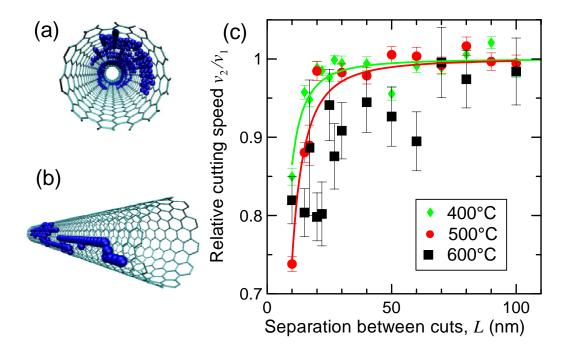
Figure 3. Results of kMC simulations. (a) Trajectory of an interstitial inside a (10,10) nanotube at  $T=500^{\circ}$ C during 30 nanoseconds. (b) Trajectory of an adatom at  $T=500^{\circ}$ C during 1 millisecond. Note the difference in the time scale. (c) Relative velocity for the second cut as obtained by the kMC simulations as a function of the separation between the cuts. Solid lines show the theoretical curves obtained through Eq. (5) at different temperatures
