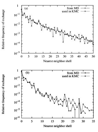
FIG. 4. Comparison between the distribution of atomic relocations calculated by MD, (lumped into the discrete jumps on a fixed fcc lattice), and the ones actually used in the KMC simulations: (a) 1 MeV Kr and (b) 62 keV He.
