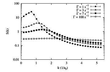
FIG. 6. Structure factor for the microstructures shown in Fig. 5, plus a curve for a high frequency of random relocations  $\Gamma = 100 \text{ s}^{-1}$ , corresponding to a solid-solution microstructure.
