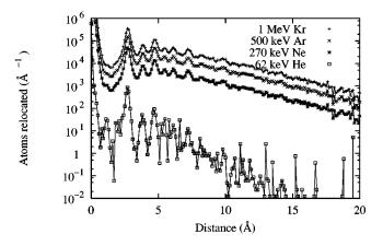
FIG. 2. Atomic relocations produced by the collision cascades initiated by the indicated ions on a  $Ag_{50}Cu_{50}$  alloy.
