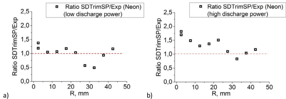
**Fig. 8.** Ratio between SDTrimSP-calculated and experimentally obtained sputtering yields for Ne -> W experiments radial distribution. a) “Low” discharge power case,  $U_b = 165$  V, experiment 4 (see Table 1); b) “High” discharge power case,  $U_b = 165$  V, experiment 4 (see Table 1).
