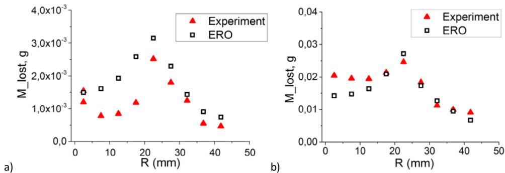
Fig. 6. Weight loss values obtained from the Ar experiment and with the ERO simulations. a) “Low” discharge power case,  $U_b = 150$  V, experiment 3 (see Table 1); b) “High” discharge power case,  $U_b = 150$  V, experiment 2 (see Table 1).
