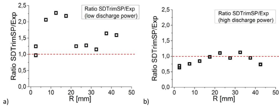
**Fig. 7.** Ratio between SDTrimSP-calculated and experimentally obtained sputtering yields for Ar -> W experiments radial distribution. The redeposition of the impurities is counted out from the experimental yield based on the ERO calculations. a) “Low” discharge power case,  $U_b = 150$  V, experiment 3 (see Table 1); b) “High” discharge power case,  $U_b = 150$  V, experiment 2 (see Table 1).
