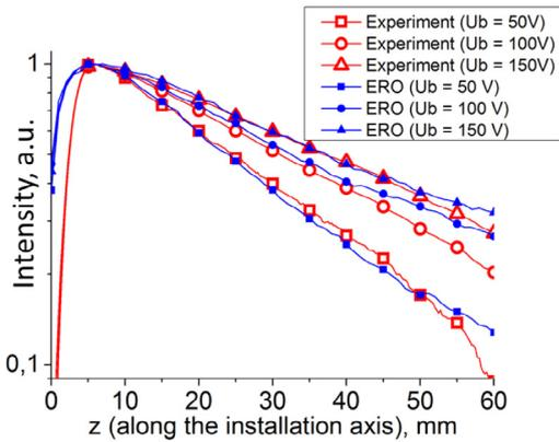
**Fig. 10.** Axial WI ( $\lambda = 400.9 \text{ nm}$ ) intensity profiles (normalized) – Ar experiment and ERO simulations. “Low” discharge power,  $U_b = 50\text{--}150 \text{ V}$ , experiment 1 (see Table 1).
