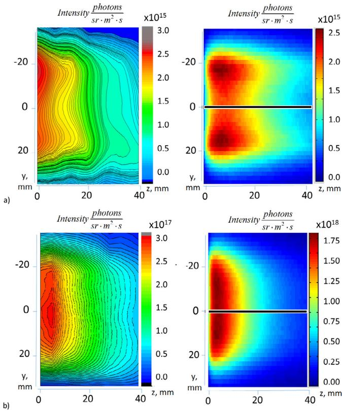
**Fig. 9.** 2D emission intensity patterns ( $\lambda = 4009 \text{ \AA}$ ) obtained in the Ar experiment with the spectrometer (left) and calculated with ERO (right). Black line – direction of axial intensity profiles extraction. a) “Low” discharge power case,  $U_b = 150 \text{ V}$ , experiment 3 (see Table 1); b) “High” discharge power case,  $U_b = 150 \text{ V}$ , experiment 2 (see Table 1).
