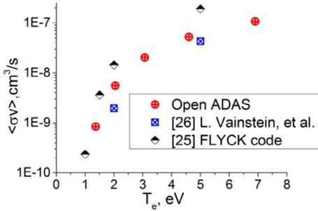
Fig. 5. Ionization data from various information sources.
