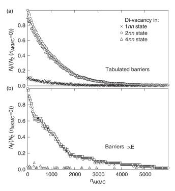
Figure 4. Occupation statistics of three bound di-vacancy states (1nn, 2nn, and 4nn) visited by one di-vacancy at each AKMC step during its diffusion migration. The di-vacancy always starts from 2nn state. The statistics was defined by 50 simulations at 300 K using (a) pre-tabulated barriers and (b) barriers from Equation (1), both with the same potential.
