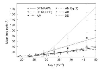
Figure 3. Mean free paths of di-vacancy against inverse temperature. The lines are guides to the eye.
