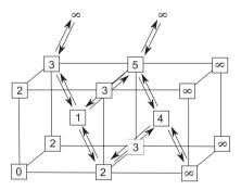
Figure 1. Different possible di-vacancy states and transitions. 0 is the position of the first vacancy; different states are obtained depending on the location of the second one.  $\infty$  positions correspond to a dissociated di-vacancy. Transitions are possible only via the exchange of the given vacancy with a nearest neighbor atom (e.g.  $1 \rightarrow 2$ ).
