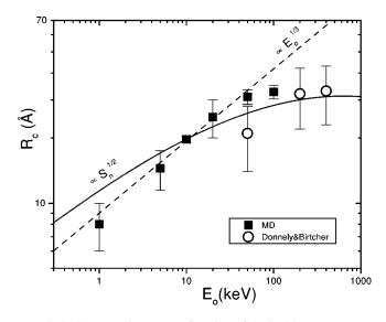
FIG. 3. Crater radius  $R_c$  as a function of the incident energy  $E_o$ , including experimental data of Donnelly and Birtcher (Refs. 10 and 35).
