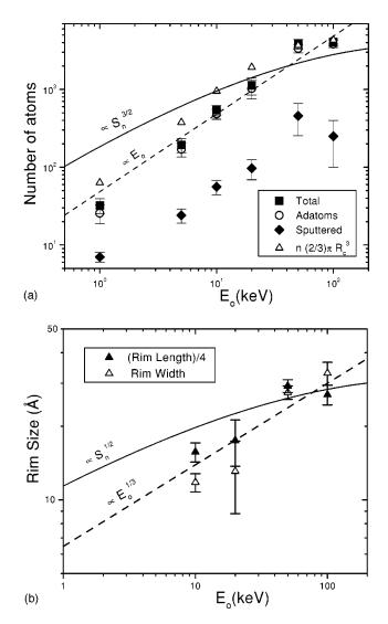
FIG. 4. (a) Total number of atoms above the surface, adatoms, and sputtered atoms as a function of the initial ion energy. Note that because many of the sputtered atoms sputter in hot clusters, and can subsequently evaporate from the cluster and redeposit on the surface, this initial sputtering yield does not exactly correspond to experimentally measured yields. (b) Crater rim length and rim width versus the initial ion energy.
